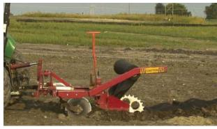
Figure 1. Static Slicing Machine
